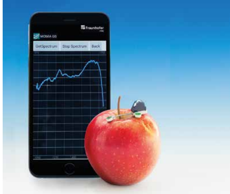
Miniaturized NIR spectrometer of Fraunhofer IPMS.
