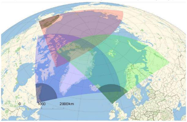
Figure D.6: Hypothetical OTH Northern Radar Coverage.
