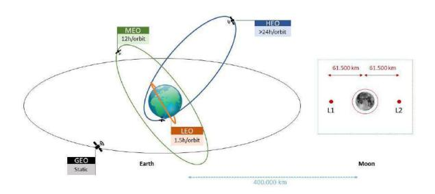
Figure J.2: LEO, MEO, GEO, HEO orbits
