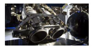
Figure H.2: SpaceX Super Draco Printed Thrust Chamber [853] (CREDIT: SpaceX)
