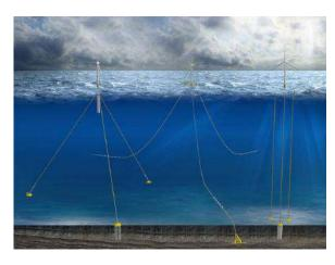
Figure F.2: Wind Platform Offshore Mooring (CREDIT: US Department of Energy)
