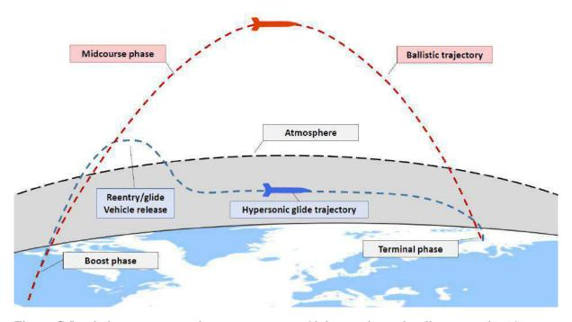
Figure G.5: Flight Trajectories of Hypersonic Boost-Glide Missiles and Ballistic Missiles (CREDIT: [741].)
