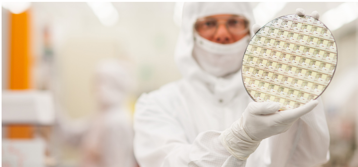
Figure 3 | A typical semiconductor wafer with chips. This thin slice of semiconductor material (e.g. silicon) is used for the fabrication of electronic chips.
