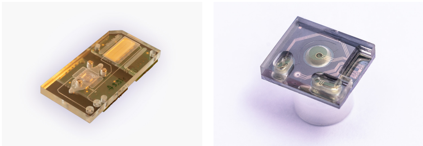
Figure 16 | Projects in which the imec microfluidic 'packaging' integration expertise was used. Left: die-to-die assembled demonstrator for detection of heart rate failure by saliva (European project KardiaTool, funded by the European Union's Horizon 2020 research and innovation program under grant agreement No 768686). Right: wafer-level packaging of sensor that measures water quality.
