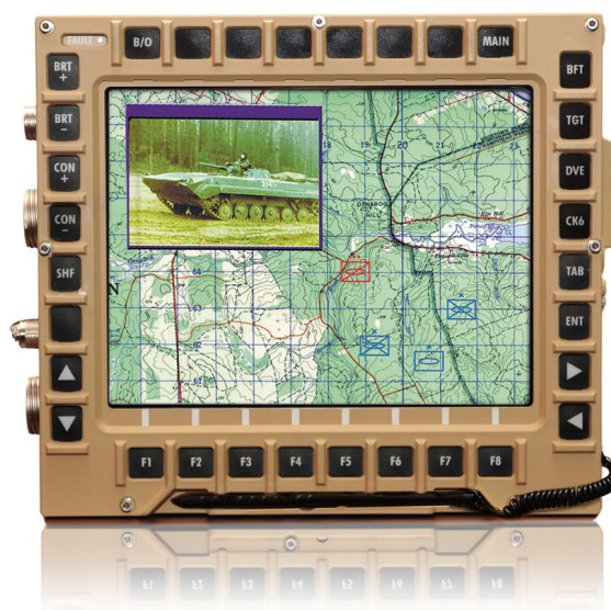
Abb2: The 10.4-inch SD7310 smart display from General Dynamics Canada is used in avionics applications. Quelle: http://www.gd-ms.ca/
