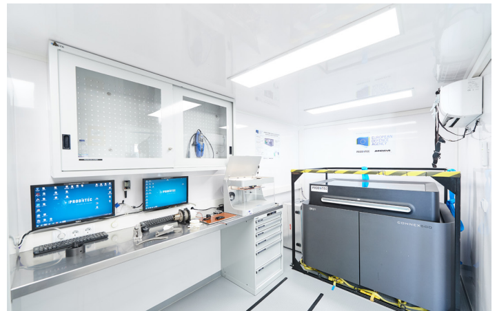
Figure 3: The interior of the EDA 3D-printing Lab, including two AM machines, post-processing, storage, and working/design area. © Source EDA
