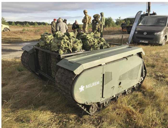
Figure 1: MILREM's TheMIS modular unmanned ground vehicle (source: MILREM)
