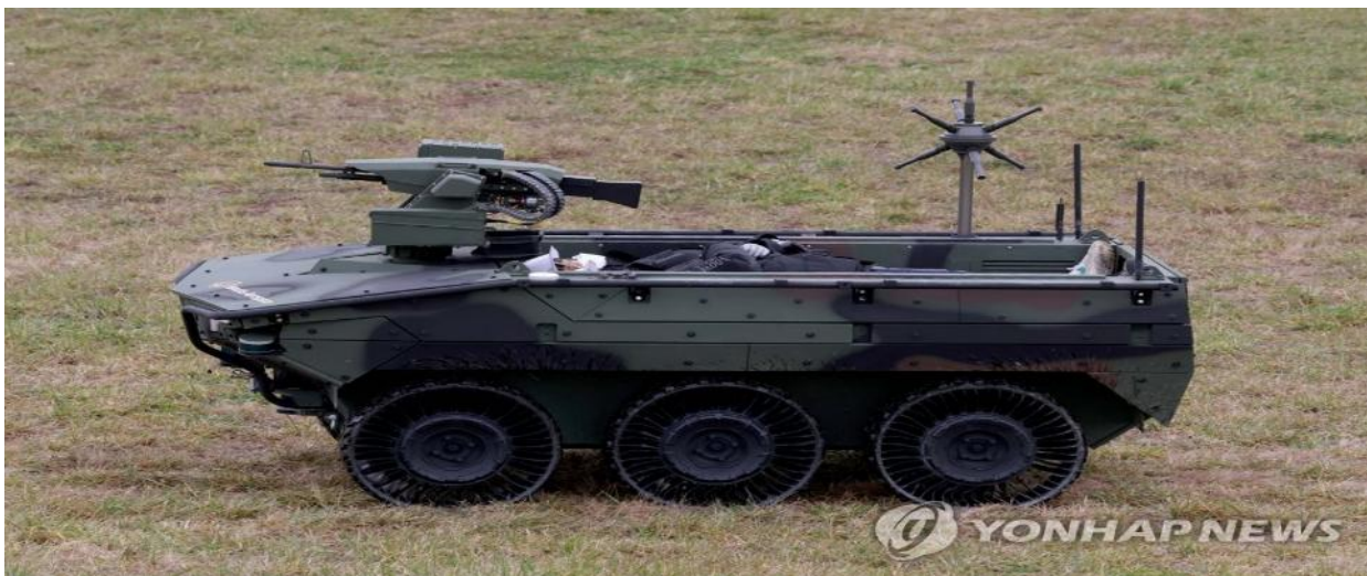
Figure 2: Hanwha's ARION-SMET multipurpose UGV. Source: Yonhap News
